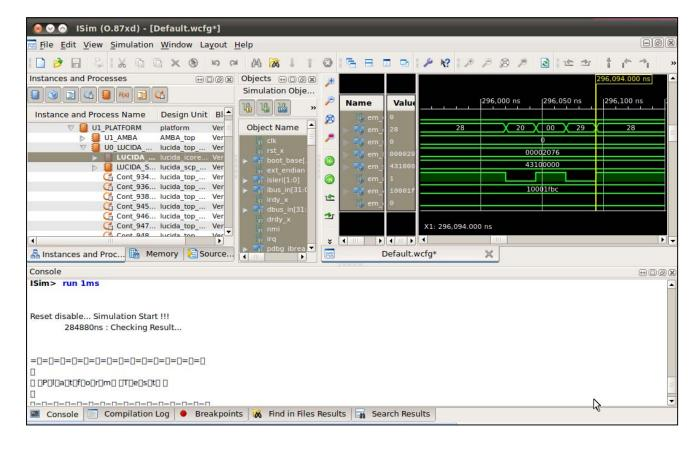
Dhrystone simulation with ISIM: The difference in hardware is an increase of DSPM (Data Scratchpad Memory) size to 32KB (the previous platform had a 8KB DSPM) and software (spsram\_16kx32\_Ben\_init.mif).
