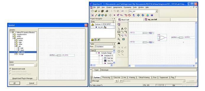
12. Connect the input pins to the xor gate inputs and the xor output to the output pin
